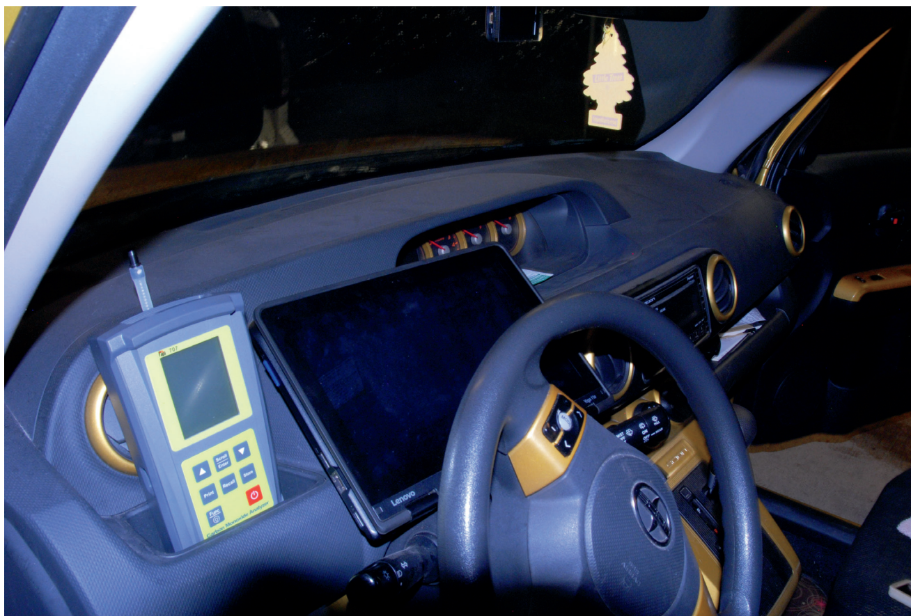
Image 2: Laptop and carbon monoxide monitor used by decedent to record carbon monoxide levels inside the vehicle.
